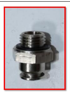
What are the differences? :-Air filter screen is not present below the Push fit assembly (after thread finished). Part no.is different .observed harness connector Loosed . ASOV screw material is different . Push fit connector shape is dissimilar.
