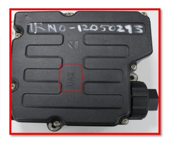
What are the differences? :- Eco fit Not mentioned on top cover. SS Screw material is used . Top cover part no.is not available inside
