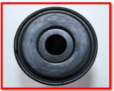
What are the differences? :- Part no. and serial no. not present on front view of damper and damper front view shape and inner view looks diverse; extra grove is available and hole size also slightly bigger. Strainer material also visually looks different.
