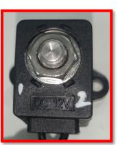
What are the differences? :- ED100% W4 is mentioned instead of W2. Serial no not available. DC12 V is written on top side. Plunger stud has over length and assembly and material looks different; sheet metal is present on assembly body instead of plastic. Number circle is not available on body
