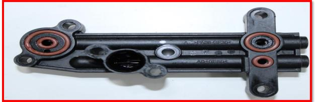
What are the differences? :- A>PA66-GF30< is mentioned instead of B>PA66-GF30< and 2 is mentioned on top side of Manifold instead of 1
