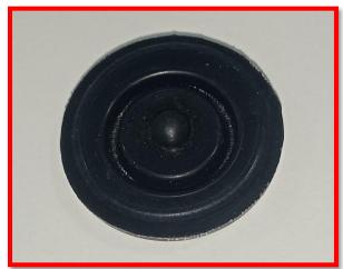
What are the differences? :- Blackish mark on check valve and shining also low. Inner shape of diaphragm is different and hardness also slightly more due to material may change.
