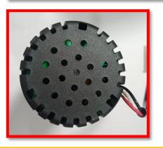
What are the differences? :- No symbol available on PCB covered body. Part no and Fluid IN arrow marks not present on read valve side metal plate. overtighten marks on below 1st screw mounting surface. No part no and numbers clocks available on plastic body of Pump in between 3 screw mounting passage (from Top View)
