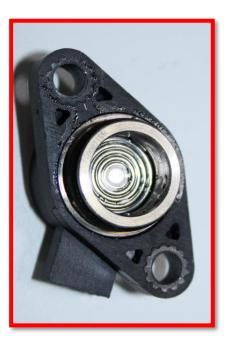
What are the differences? :- Barcode and part no is changed. Circles present inside the sensing element of pressure sensor are differently designed.
