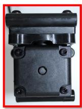
What are the differences? :- Barcode, Part no. and scan bar is dissimilar. Covered Rotating shaft area from RH side view and bottom view of pump (manifold fitment side) and not visible
