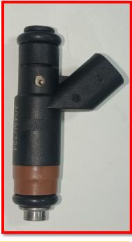
What are the differences? :- DEKA name is not available and sr no. series is different. And Part no/sr.no font is dissimilar. Nozzle tip is diverse and spray hole size is bigger than genuine doser. Rupture marks found on back side of MV (plastic surface)
