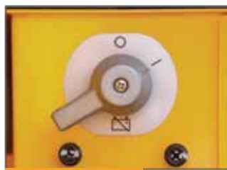
BATTERY DISCONNECT SWITCH
