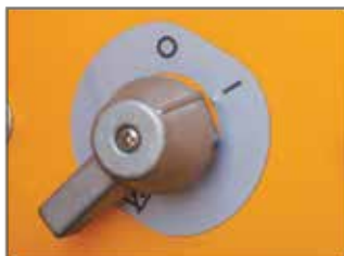
BATTERY DISCONNECT SWITCH
