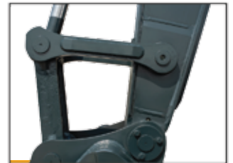
Reinforced bucket link
