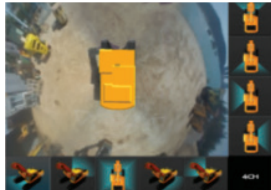
AAVM (Advanced Around View Monitoring) Camera System (Option)
