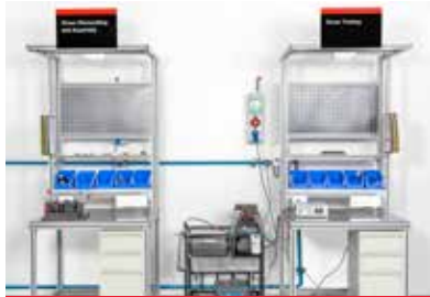
Aftertreatment service station
