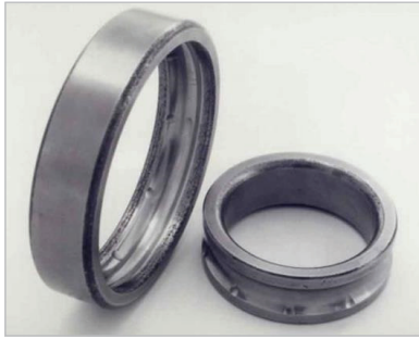
Figure 1 - Brinelling - Static Deformation of Metal Race and Wear Marks at Interface of Balls and Race
