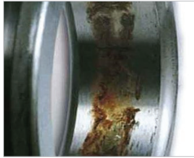
Figure 2 - Fretting – Scoring, Corrosion, Discoloration
